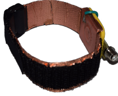
Figure 9: Velcro wrist strap covered in conductive copper tape used to couple the SDR receiver to the body.
