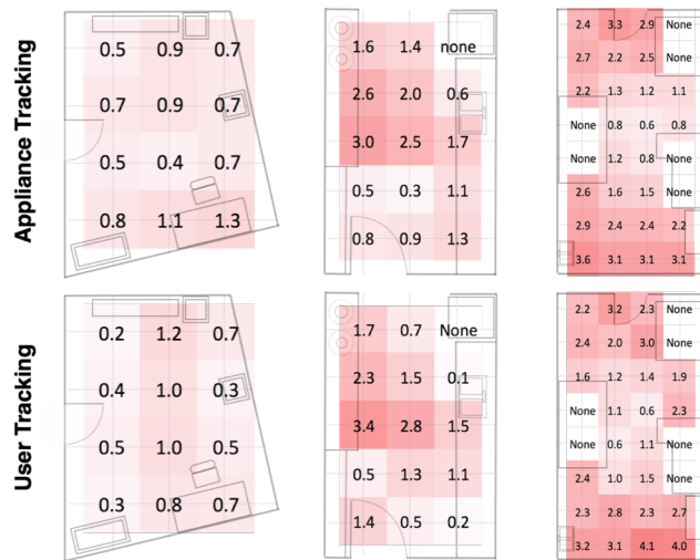
Figure 12. Tracking distance error at our three test locations. Left to right: office, kitchen and workshop.
